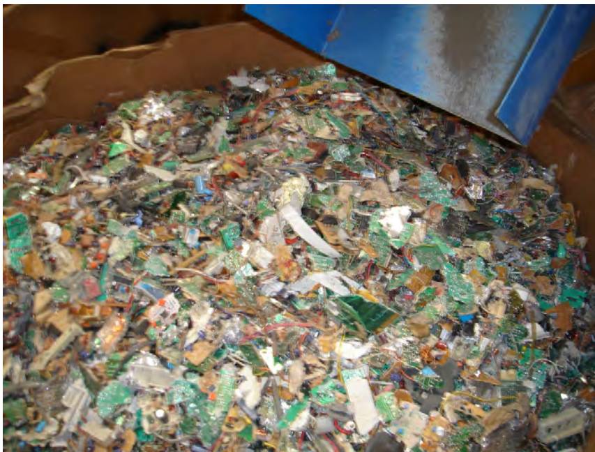
Picture 4: This is circuit board without aluminum or any other metals. It is then sent through another sorter to sort plastics out.
