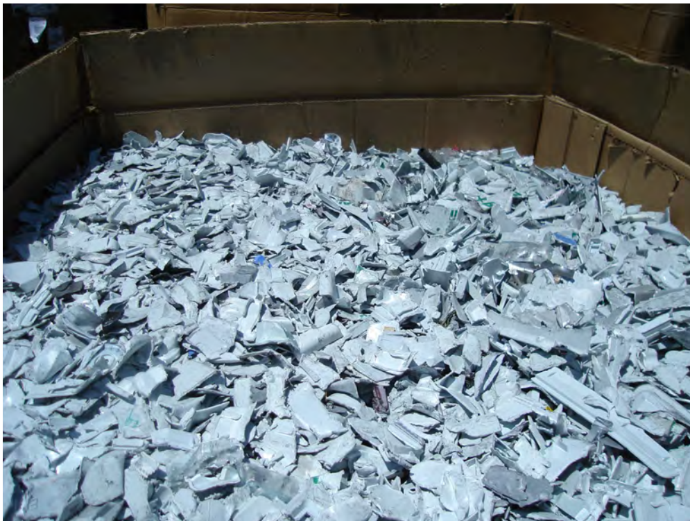
Picture 6: ABS plastics are separated from the electronics. Plastic seen here are from printers, fax machines, scanners, and computer monitor housing.
