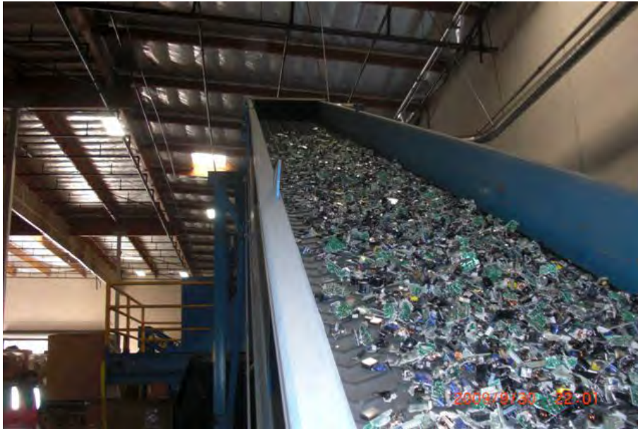
Picture 5: Here shredded electronics are moving along the belt to be further separated.
